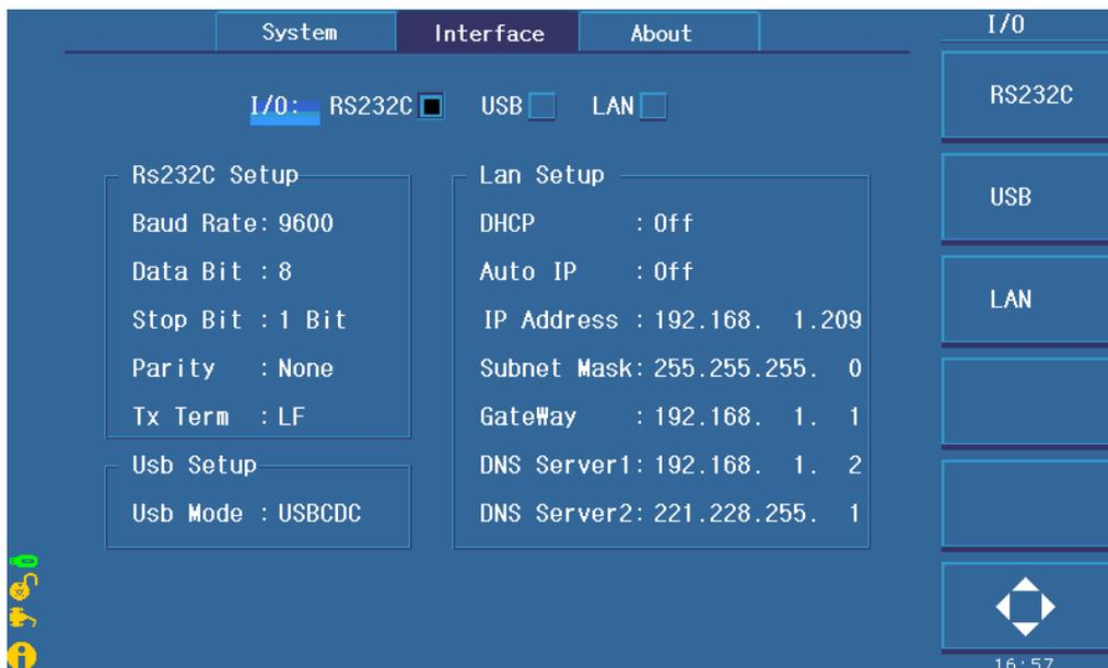
Figure 6-9 Network parameters of ST2883
